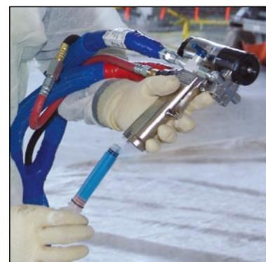
Each cartridge contains about 1,500 trigger shots (pulls) a day, allowing you to work through one to two kits.
